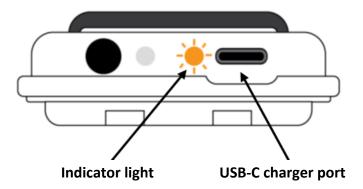
**Low Battery:** When the orange light flashes twice every 30 seconds, the battery is below 15%. Typical battery life is 9 hours.
