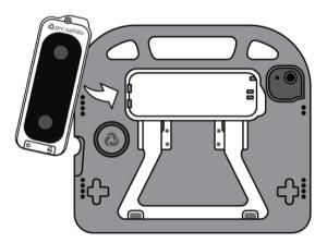
3. On the right side, secure the speaker with the screw that was provided with the speaker.
