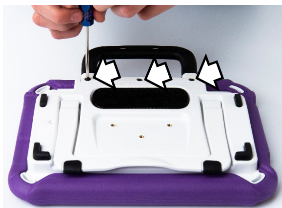
Via Mini: Remove three screws
