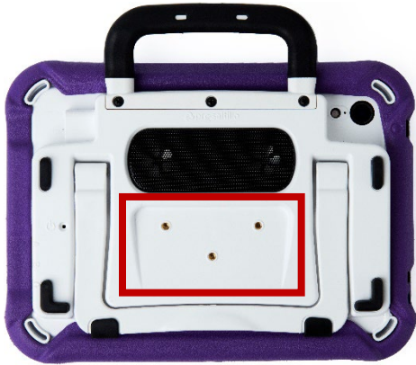
Threaded holes for attaching a mounting plate
