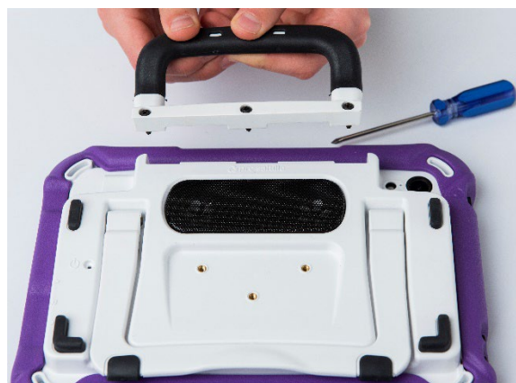
Via Mini: Remove three screws
