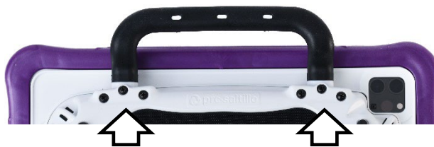
Via Pro: Remove six screws
