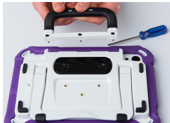
Via Mini: Remove three screws
