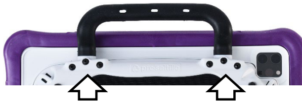
Via Pro: Remove six screws
